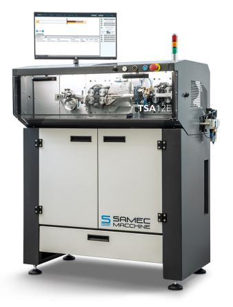
TSA12EVO is designed for the processing of insulated and uninsulated single core, multicore and flat cables. The machine counts the batch, measures the cutting length, strips and unjackets without needing to change blades. Through an easy-to-use control panel with a 12-inch color touchscreen display, the operator can constantly overview the work in progress, set and correct batch parameters, and receive batch information.
